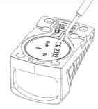
When removing the battery, always lever against the body not the terminals.
