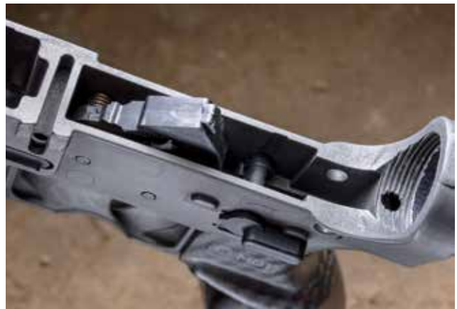
The trigger springs are metal, but the hammer is polymer. Many are hesitant to use polymer for such an important part, but it functioned without issue.
