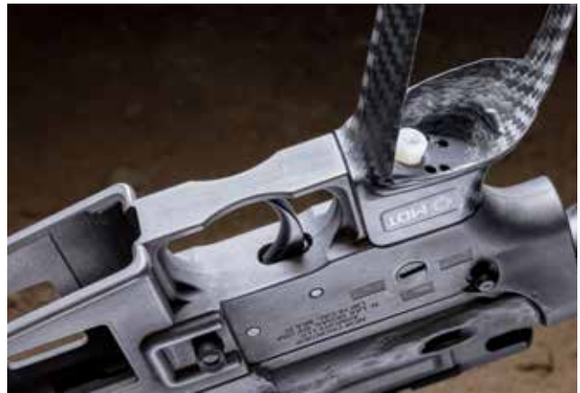
Note the screw attaching the grip to the lower receiver. It's white because its made from a strong and lightweight nylon. "Ounces make pounds," some say, but grams make ounces.
